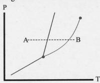
If the temperature is increased as indicated by the dotted line A-B, which of the following describes the sequence of phases that will be observed?
